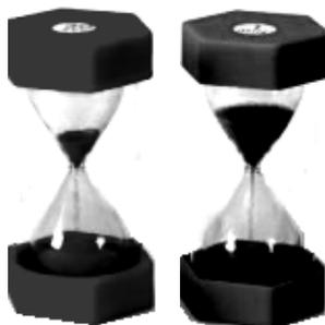
These are sand timers (also called hourglasses). The time they measure is the time it takes for the sand to fall from the top bulb, through the narrow tube, into the bottom bulb.
